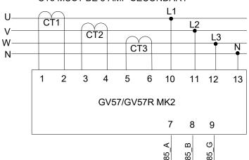
WARNING: When there is load current, C. T. secondary must not be open circuit, Otherwise, the high voltage generated will pose a danger to personal safety.
